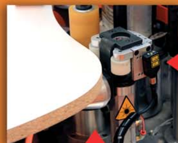
FLOATING laser follows shape geometry and position, assuring tighter joint cuts, even on bowed or large parts (patent pending)
